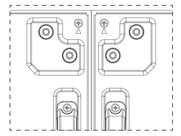
Install "Edge Alignment Kit-2" with 4 PCS of screw on outer, bigger holes.
