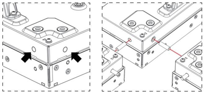
There are 8 holes on the four corners of displays designed for plug-in the edge alignment pin.
