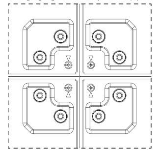
Install "Edge Alignment Kit-1" with 8 PCS of screw on outer, bigger holes.
